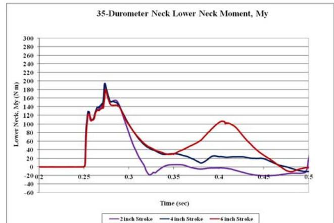
Figure 2: 35-Durometer Neck.
